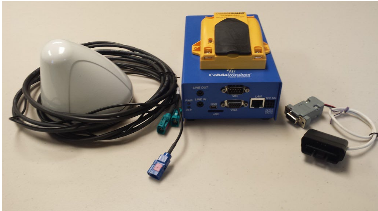
Figure 5 - Light Vehicle OBE, Antenna and Cables (Source: Synesis Partners LLC)
