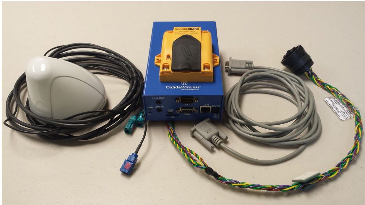
Figure 4 - Heavy Vehicle OBE, Antenna and Cables (Source: Synesis Partners LLC)
