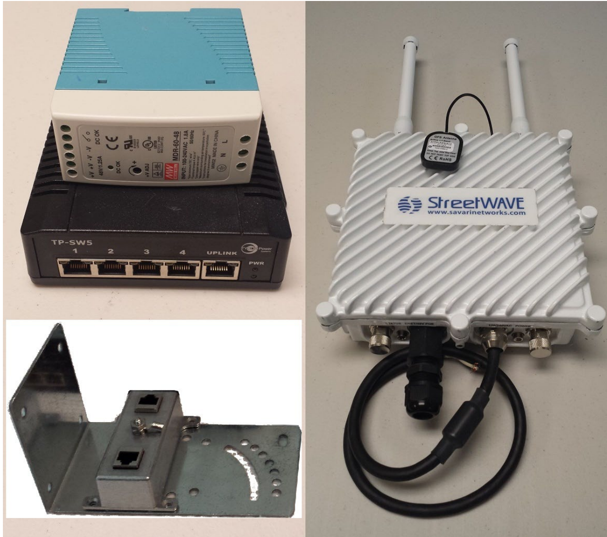
Figure 10 - RSE, Ethernet Switch, and Bracket/Surge Suppressor (Source: Synesis Partners LLC)
