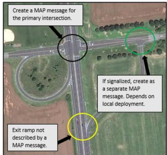
Figure 23: Aerial view of jug handle intersection
