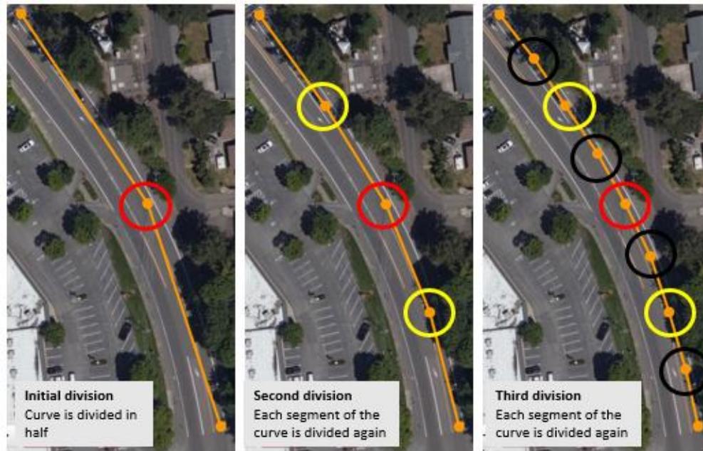
Figure 14: Node spacing in horizontal curves
