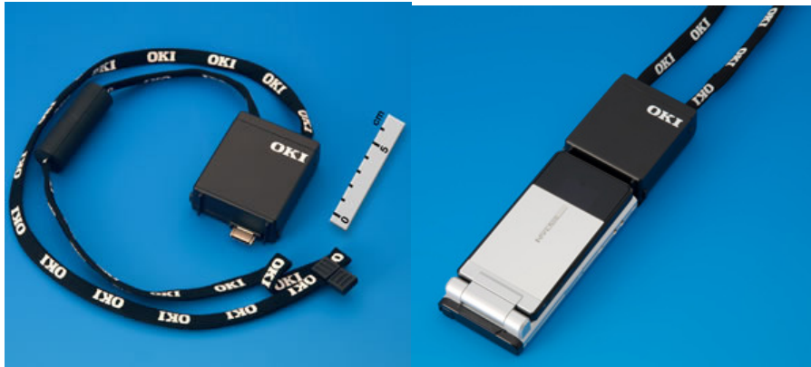
Figure 3.1 DSRC attachment for mobile phone by OKI, Japan
