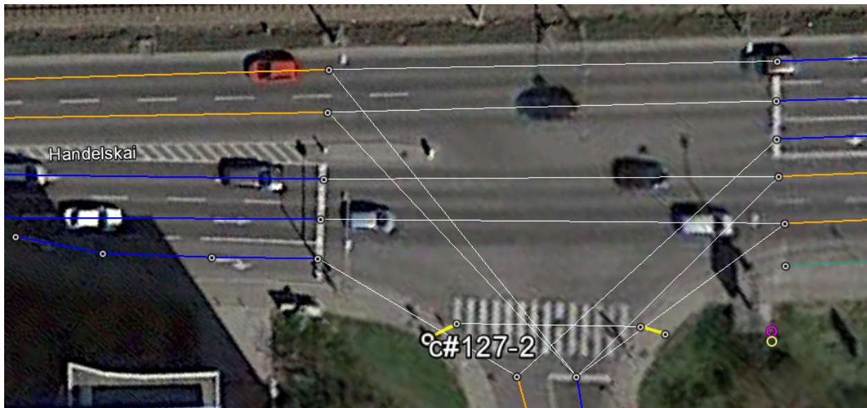
Figure 5: Zoomed in view of the intersection. Connecting lanes are indicated as straight white lines.
