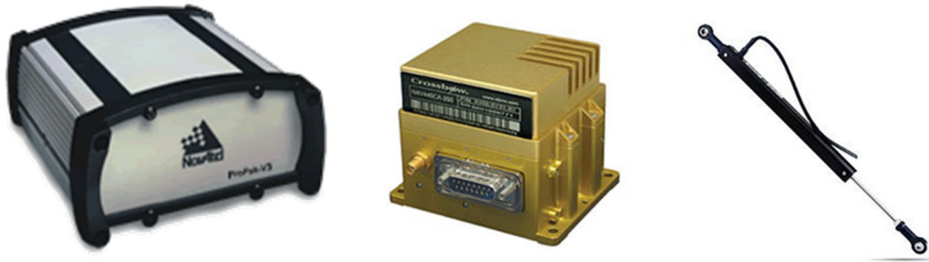
Figure 15 – Hardware used in prototype system (Left) Novatel Propak-v3 GPS receiver (Center) Crossbow 440 IMU (Right) Celesco Linear Potentiometer
