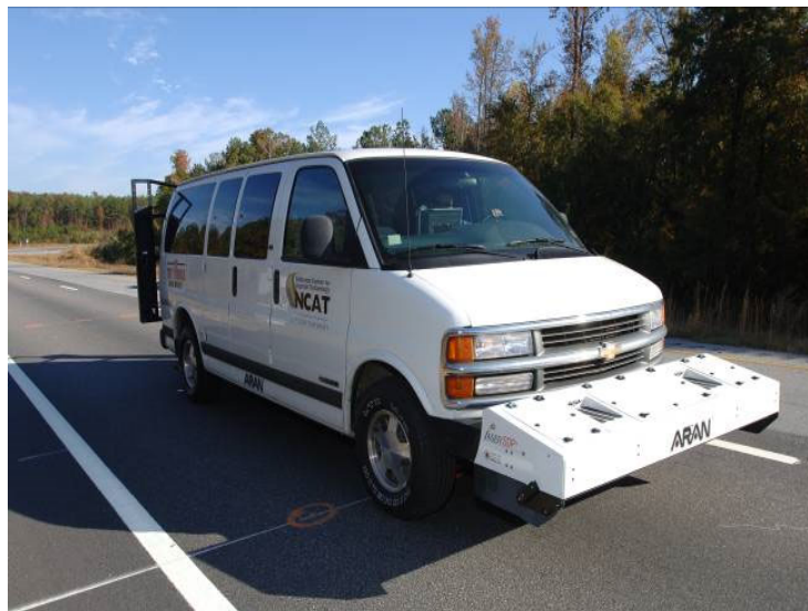
Figure 4 – NCAT van equipped with laser profilometers
