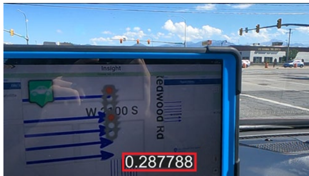
Figure 9. Video Processing Software can Add a Relative Timestamp to Video to Facilitate Analysis, as shown in the Red Box.
