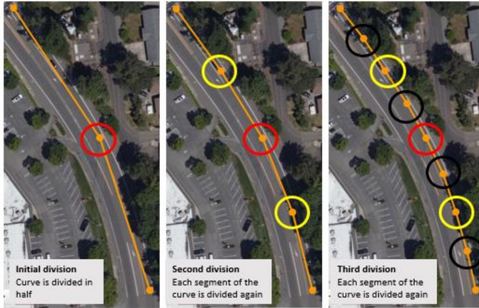
Figure 13: Node spacing in horizontal curves
