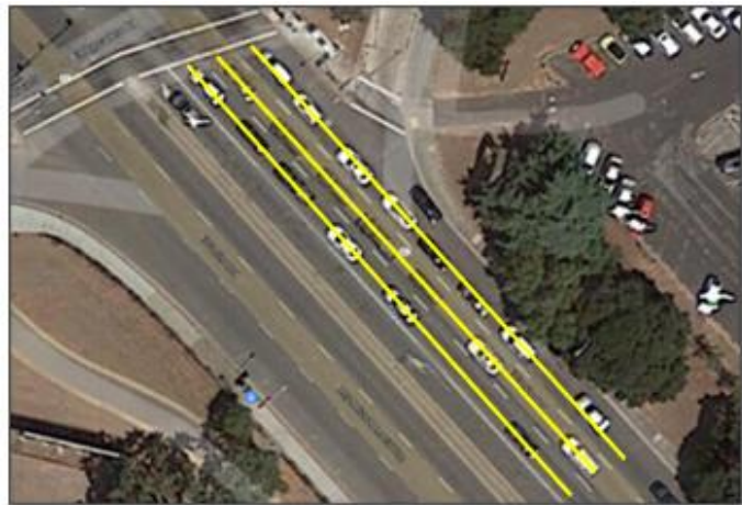
Figure 5: Yellow line overlaid on three straight parallel ingress lanes that match criteria for computed lanes Map source: Google Maps, Drawing source: Athey Creek Consultants
