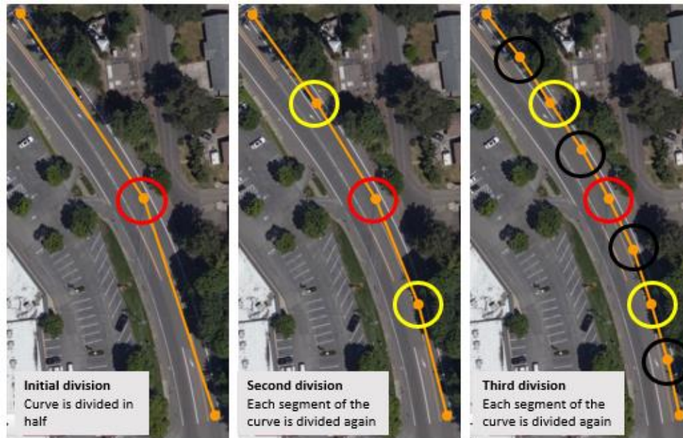
Figure 13: Node spacing in horizontal curves
