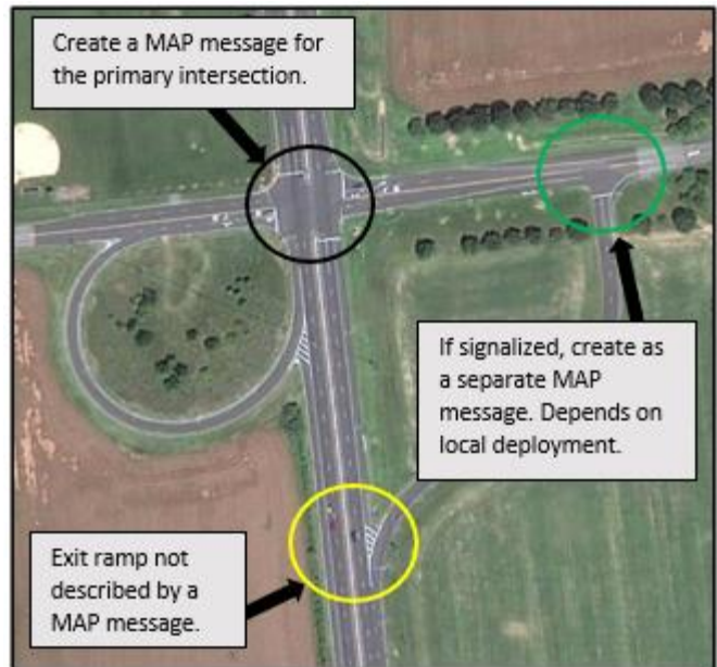
Figure 22: Aerial view of jug handle intersection Map source: Google Maps, Drawing source: Athey Creek Consultants
