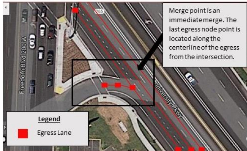
Figure 17: Example egress node placement for an intersection where the merge point is an immediate merge. Map source: Google maps, Drawing source: Athey Creek Consultants
