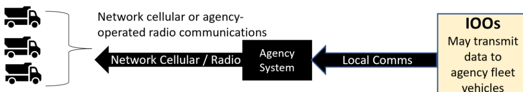
Figure 7: Illustration of IOO to vehicle data path #3: an IOO internal CV data communication to fleet vehicles
