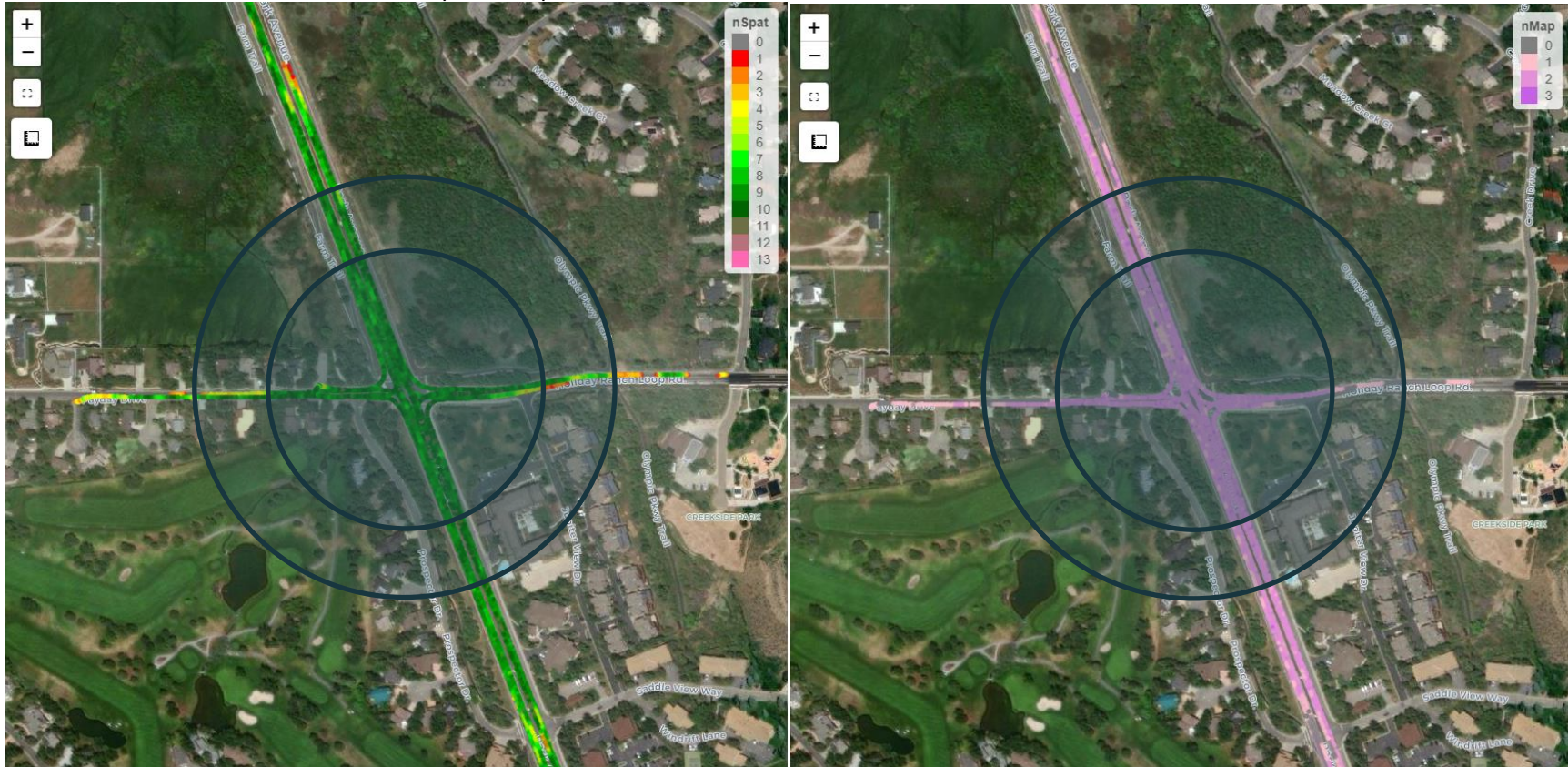
40 mph (NB/SB) and 25 mph (WB/WB) minimum reception ranges are represented by the outer and inner blue circles, respectively.
