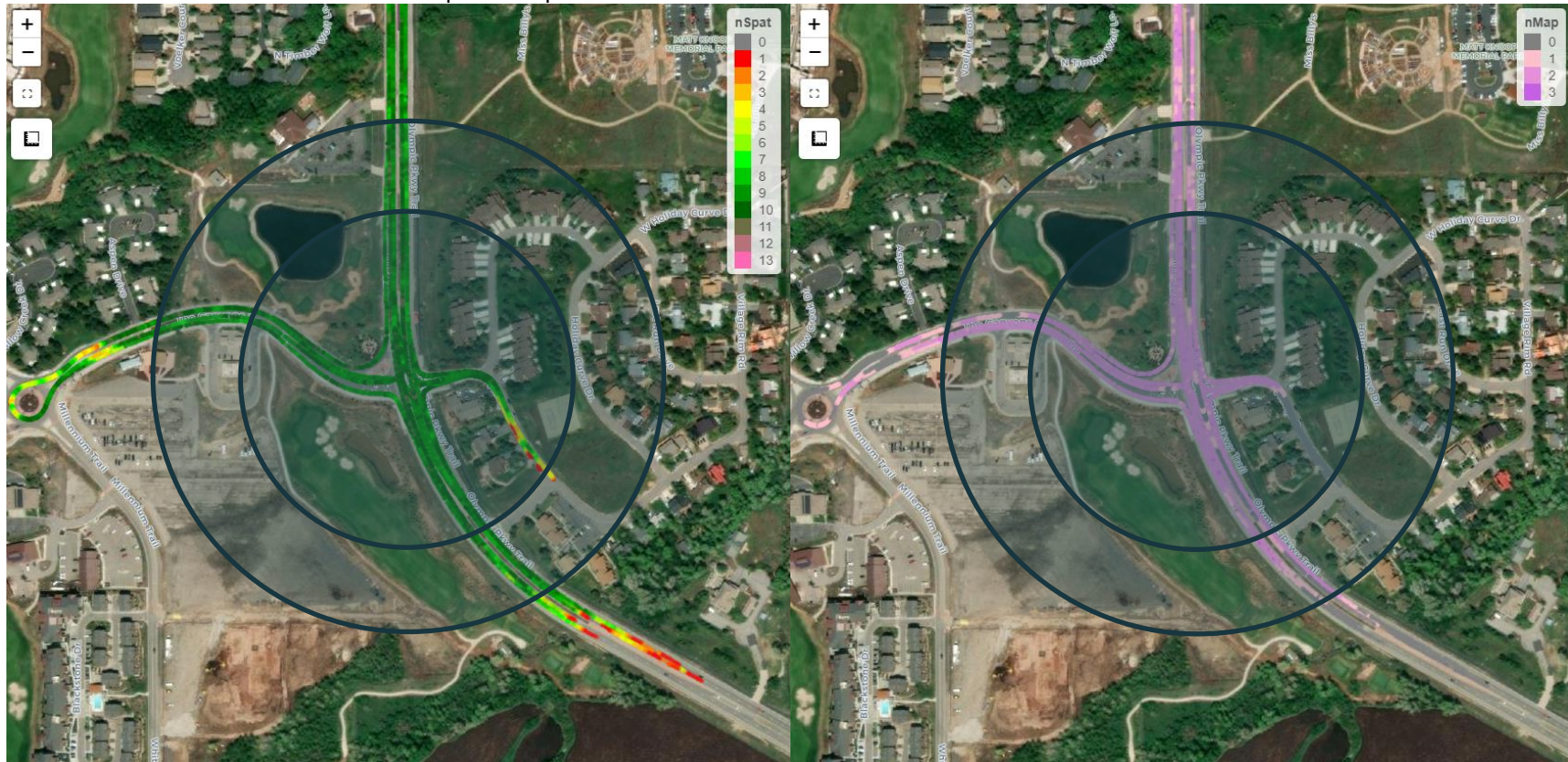
45 mph (NB/SB) and 25 mph (EB/WB) minimum reception ranges are represented by the outer and inner blue circles, respectively.
