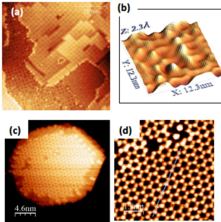
**Figure 1:** (a) NiO thin film on Ni 14%Cr alloy surface, (b) Graphene layer on a Cu-substrate – the deformation of the graphene layer is caused by  $C_{60}$  molecules inserted between Cu and graphene, (c)  $MoSi_2$  crystallite with a silicene top layer, (d) high resolution image of the silicene layer with atomic resolution.
