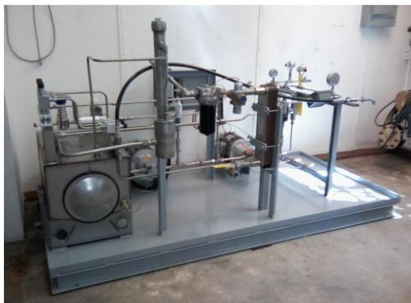
Fig. 9 Oil-gas mixture supply system for the seal test rig
