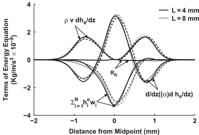
**Figure 15** Comparison of the terms in quasi one-dimensional energy equation using axisymmetric (OpenFOAM—solid line) and quasi one-dimensional (dashed line) simulations, for two separation distances using 6.5 mm nozzles (i)  $L = 8$  mm and strain rate of  $a = 290$   $\text{s}^{-1}$  and (ii)  $L = 4$  mm and strain rate of  $a = 354$   $\text{s}^{-1}$ . The residue of axisymmetric solution is identified as  $R_h$ , which is mainly due to the radial heat conduction term.
