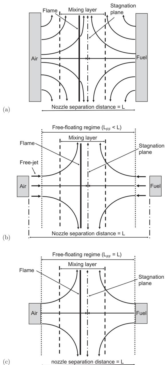
**Figure 1** Schematic of counterflow diameter and separation distance effects: (a) large nozzle setup (Seshadri type burner) with plug-flow velocity profile, (b) small diameter nozzles with non-ideal separation distances ( $L > L_{FF}$  with plug flow and free-jet or  $L < L_{FF}$  with finite  $U$  values), and (c) small nozzles with ideal separation distance ( $L = L_{FF}$ ).
