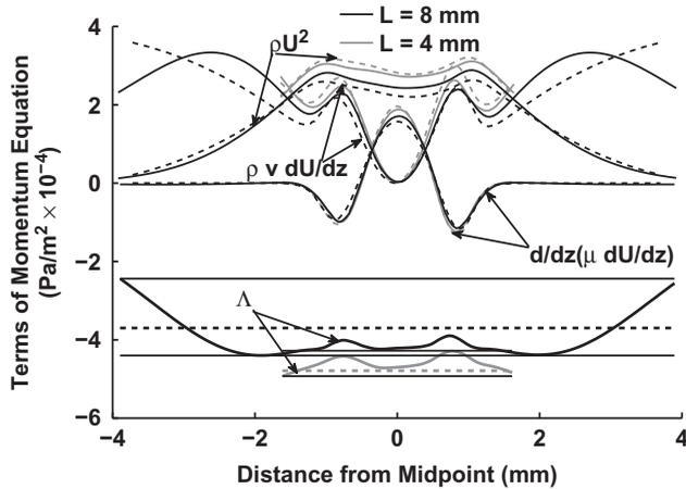
**Figure 14** Comparison of the terms in radial momentum equation (including eigenvalue,  $\Lambda$ ) using axisymmetric (OpenFOAM—solid line) and quasi one-dimensional (dashed line) simulations, for two separation distances using 6.5 mm nozzles (i)  $L = 8$  mm and strain rate of  $a = 290$   $\text{s}^{-1}$  and (ii)  $L = 4$  mm and strain rate of  $a = 354$   $\text{s}^{-1}$ .
