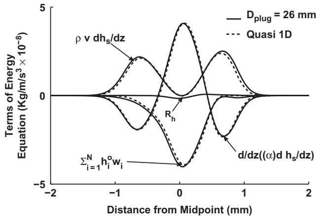
**Figure 6** Comparison of the terms in the quasi one-dimensional energy equation using axisymmetric (OpenFOAM—solid line) and quasi one-dimensional (dashed line) simulations, for a plug flow with a diameter of 26 mm (Seshadri type burner) and strain rate of  $a = 375 \text{ s}^{-1}$ . The residue of axisymmetric solution is identified as  $R_h$ , which is mainly due to the radial heat conduction term.
