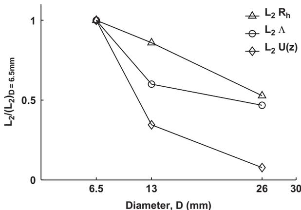
**Figure 16** Comparison of the  $L_2$ -norm evaluated based on  $\Lambda$ ,  $R_h$ , and  $U$  as a function of the nozzle diameter, for nozzle separation distance of  $L = 4$  mm. *Note:*  $L_2$ -norm values are normalized by those at  $D = 6.5$  mm.
