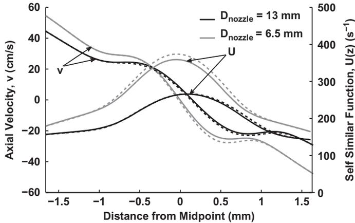
**Figure 7** Comparison of axial velocity and self-similarity function ( $U(z)$ ) using axisymmetric (OpenFOAM—solid line) and quasi one-dimensional (dashed line) simulations, for (i) nozzle flow with diameter of 13 mm and strain rate of  $a = 268 \text{ s}^{-1}$ , and (ii) nozzle flow with diameter of 6.5 mm and strain rate of  $a = 354 \text{ s}^{-1}$ .
