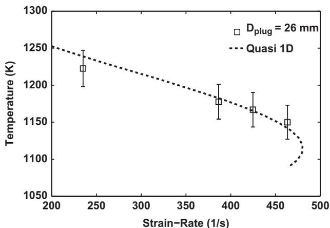
**Figure 21** Prediction of maximum flame temperature variation with increasing flow strain rate of a diluted non-premixed hydrogen vs. air flame, using both OpenFOAM and quasi one-dimensional simulations.
