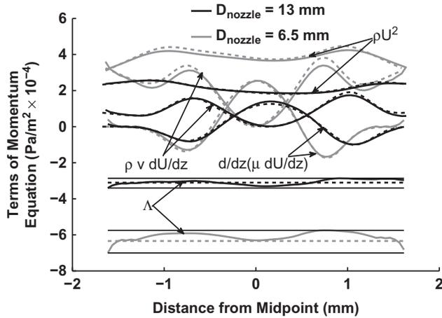
**Figure 9** Comparison of the terms in radial momentum equation (including eigenvalue,  $\Lambda$ ) using axisymmetric (OpenFOAM—solid line) and quasi one-dimensional (dashed line) simulations, for (i) nozzle flow with diameter of 13 mm and strain rate of  $a = 268 \text{ s}^{-1}$  and (ii) nozzle flow with diameter of 6.5 mm and strain rate of  $a = 354 \text{ s}^{-1}$ .
