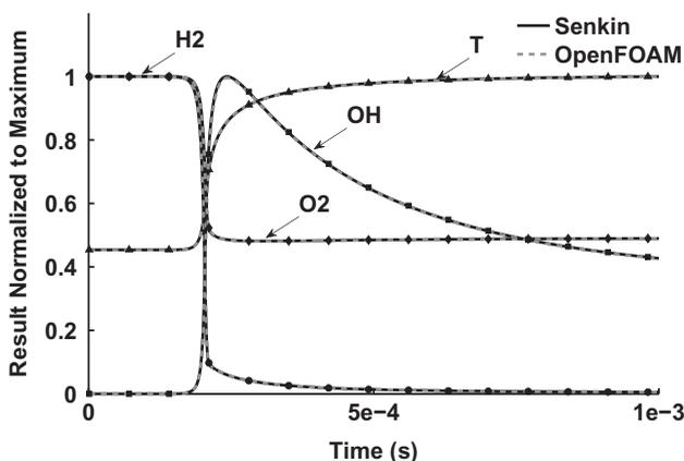
**Figure 18** Comparison of temperature and species evolution of a homogeneous mixture at constant pressure and constant enthalpy conditions using OpenFOAM and SENKIN codes. Results are normalized to their maximum values, i.e.,  $T/T_{\max}$ ,  $X_{H_2}/(X_{H_2})_{\max}$ ,  $X_{O_2}/(X_{O_2})_{\max}$ , and  $X_{OH}/(X_{OH})_{\max}$ .
