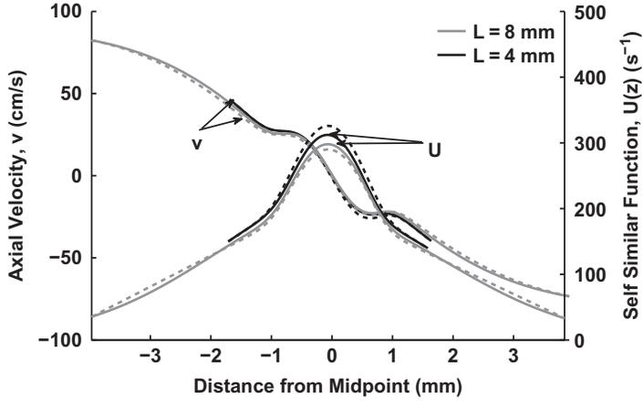
**Figure 12** Comparison of axial velocity and self-similarity function ( $U(z)$ ) using axisymmetric (OpenFOAM—solid line) and quasi one-dimensional (dashed line) simulations, for two separation distances using 6.5 mm nozzles (i)  $L = 8$  mm and strain rate of  $a = 290 \text{ s}^{-1}$  and (ii)  $L = 4$  mm and strain rate of  $a = 354 \text{ s}^{-1}$ .
