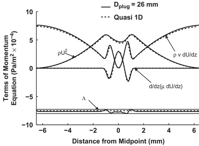
**Figure 5** Comparison of the terms in radial momentum equation (including eigenvalue,  $\Delta$ ) using axisymmetric (OpenFOAM—solid line) and quasi one-dimensional (dashed line) simulations, for a plug flow with a diameter of 26 mm (Seshadri type burner) and strain rate of  $a = 375 \text{ s}^{-1}$ .
