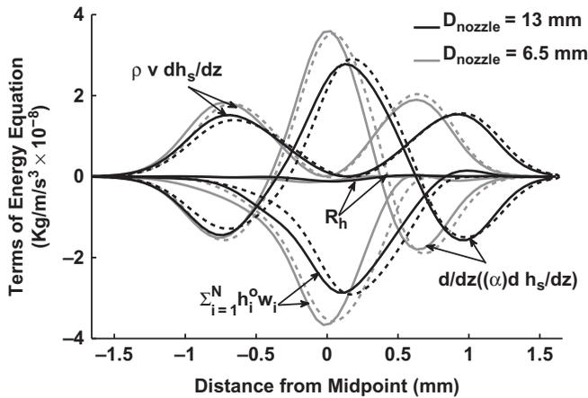
**Figure 10** Comparison of the terms in the quasi one-dimensional energy equation using axisymmetric (OpenFOAM—solid line) and quasi one-dimensional (dashed line) simulations, for (i) nozzle flow with diameter of 13 mm and strain rate of  $a = 268 \text{ s}^{-1}$  and (ii) nozzle flow with diameter of 13 mm and strain rate of  $a = 354 \text{ s}^{-1}$ . The residue of axisymmetric solution is identified as  $R_h$ , which is mainly due to the radial heat conduction term.
