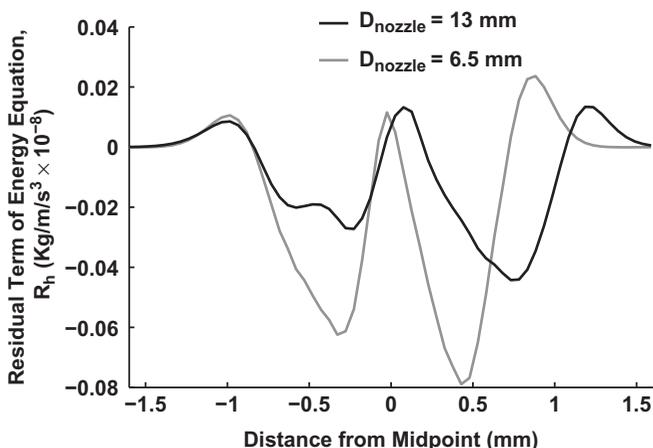
**Figure 11** Comparison of the residue term only in the energy equation ( $R_h$ ), for (i) nozzle flow with diameter of 13 mm and strain rate of  $a = 268 \text{ s}^{-1}$  and (ii) nozzle flow with diameter of 13 mm and strain rate of  $a = 354 \text{ s}^{-1}$ .
