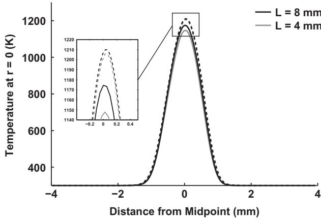
**Figure 13** Comparison of temperature using axisymmetric (OpenFOAM—solid line) and quasi one-dimensional (dashed line) simulations, for two separation distances using 6.5 mm nozzles (i)  $L = 8$  mm and strain rate of  $a = 290 \text{ s}^{-1}$  and (ii)  $L = 4$  mm and strain rate of  $a = 354 \text{ s}^{-1}$ .
