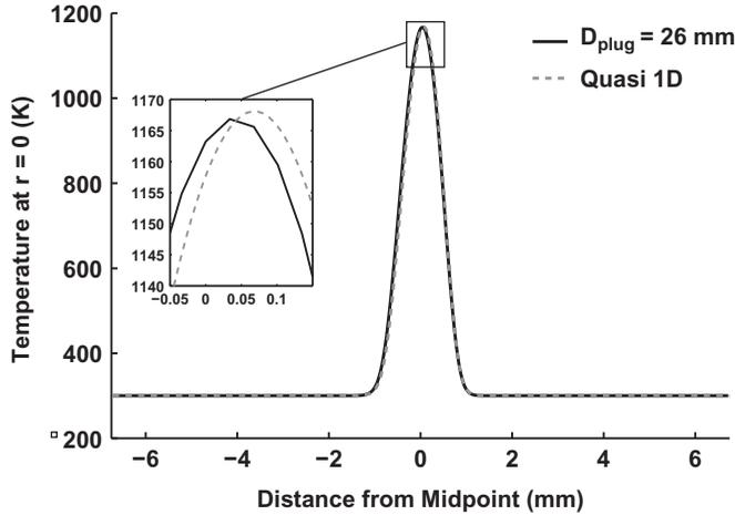
**Figure 4** Comparison of flame temperature using axisymmetric (OpenFOAM—solid line) and quasi one-dimensional (dashed line) simulations, for a plug flow case with a diameter of 26 mm (Seshadri type burner) and strain rate of  $a = 375 \text{ s}^{-1}$ .
