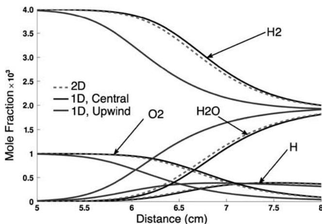
**Figure 19** Variation of species mole fractions in a one-dimensional reactor at constant  $T = 980$  K and  $p = 1$  atm, with inflow conditions of  $v = 2$  m/s,  $X_{H_2} = 0.004$ ,  $X_{O_2} = 0.001$ , and  $X_{N_2} = 0.995$ .
