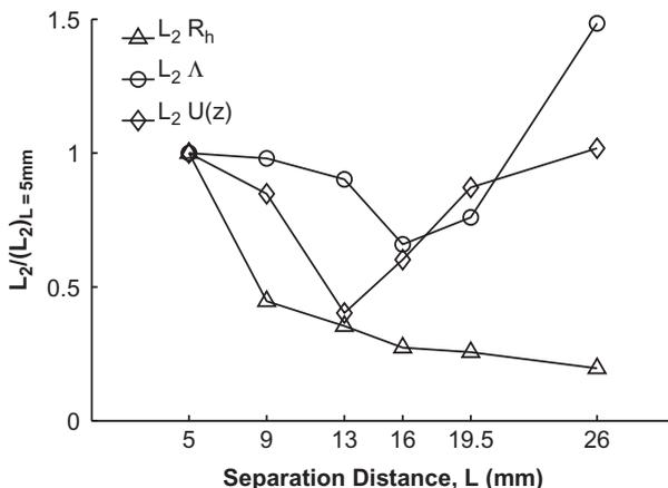
**Figure 17** Comparison of the  $L_2$ -norm evaluated based on  $\Lambda$ ,  $R_h$ , and  $U$  as a function of the nozzle separation distance, for nozzle diameter of  $D = 13$  mm. *Note:*  $L_2$ -norm values are normalized by those at  $L = 5$  mm.
