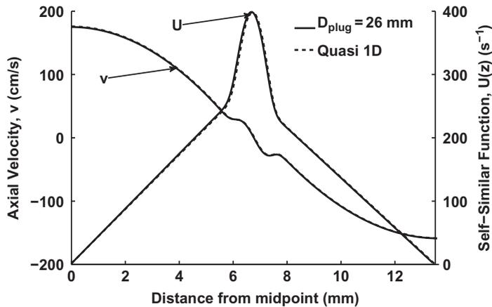
**Figure 3** Comparison of axial velocity and self-similarity function ( $U(z)$ ) using axisymmetric (OpenFOAM—solid line) and quasi one-dimensional (dashed line) simulations, for a plug flow case with a diameter of 26 mm (Seshadri type burner) and local strain rate of  $a = 375 \text{ s}^{-1}$ .
