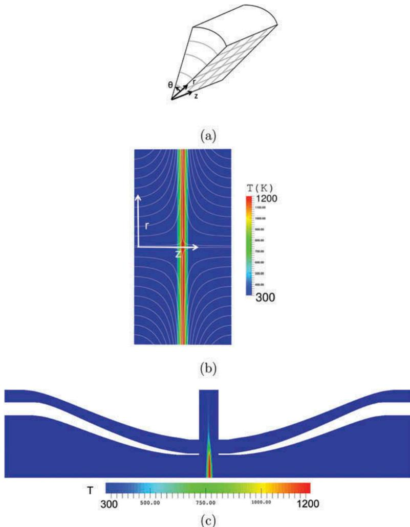
**Figure 2** Computational domains implemented showing (a) 2D wedge-shape mesh with  $r$  and  $z$  coordinates, (b) typical solution from large diameter Seshadri type plug-flow burners, and (c) solution from a small diameter nozzle type burners.
