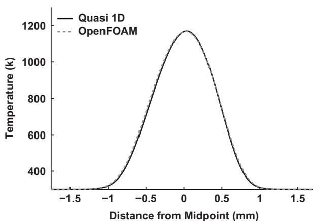
**Figure 20** Comparison of the flame temperature profiles predicted using OpenFOAM and quasi one-dimensional codes, for strain rates of  $a = 375 s^{-1}$ .
