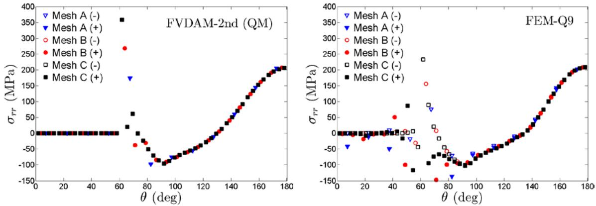
Radial stress distributions around the fiber/matrix interface of a unidirectional metal/matrix composite reinforced by ceramic fibers with a partially debonded interface subjected to transverse tension, illustrating superior traction continuity satisfaction of the generalized FVDAM theory relative to the finite-element method. (Source: Cavalcante, M.A.A, Pindera, M.-J., Generalized FVDAM theory for elastic-plastic periodic materials. *Int. J. Plasticity* 77 (2016) 90-117.)
