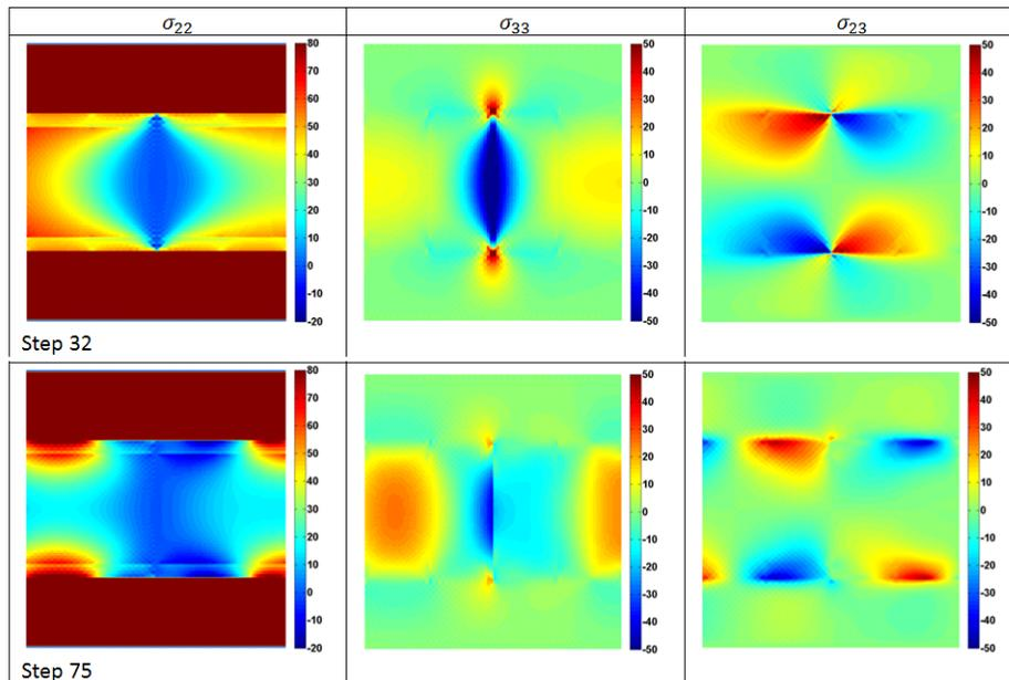
Simulation of damage evolution in cross-ply composite laminates using our finite-volume based homogenization approach, illustrating “on the fly” for the first time damage mode bifurcation from transverse cracking of the inner 90 deg plies to delamination of the 0/90 deg ply interface. (Source: Tu, W. and Pindera, M-J., **Damage evolution in cross-ply laminates revisited via cohesive zone model and finite-volume homogenization. Composites Part B 86, (2016) 40-60.**)
