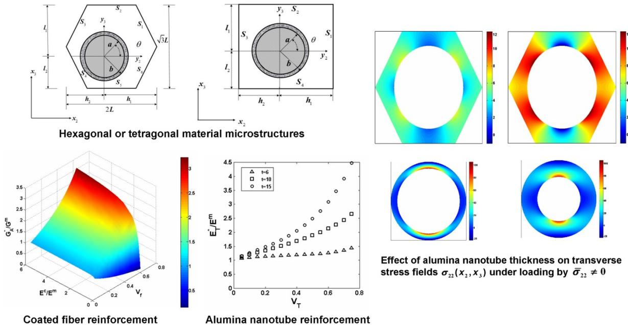
Using our locally-exact homogenization theory, a user with minimal mechanics exposure can rapidly investigate the effect of coatings on homogenized moduli of both coated fiber composites as well as hollow nanotubes. (Source: Wang, G. and Pindera, M.-J., Locally-exact homogenization of unidirectional composites with coated or hollow reinforcement. *Materials and Design* 93 (2016) 514–528.)
